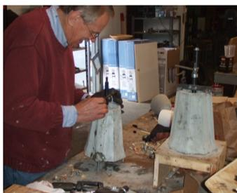
The initial concept for developing a mini-Sheller was to create a smaller, cheaper machine to shell smaller seeds such as coffee and neem. It is currently in an experimental phase in Tanzania being tested on coffee beans and in India for shelling neem (used as a natural repellent and
